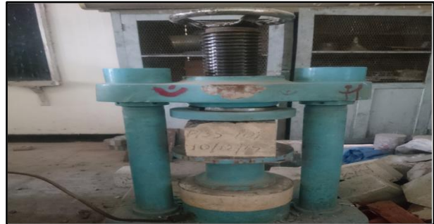
Fig4: During Compression Test of the Cubes TableVI: Sieve Analysis of Fine Aggregate
